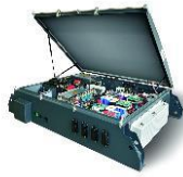
Roof container of traction and wiring harness equipment
