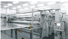
"Optimized interface between electrical and mechanical systems" Film stretching line in detail , © Brückner Group)
